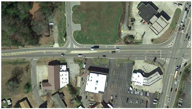
Figure 27: Example of Access Management on US-411 near SR-77 Intersection
