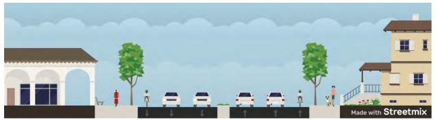
Figure 25: Complete Street Cross Section – Town Center Arterial
