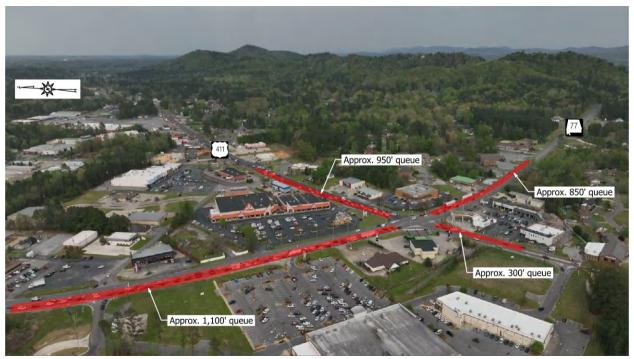
Figure 6: PM Peak Hour Drone Observations
