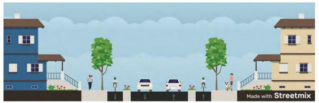
Figure 23: Complete Street Cross Section – Rural/Suburban Collector
