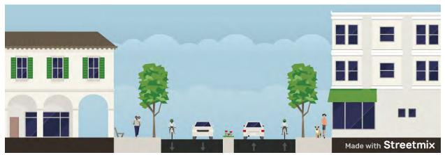
Figure 26: Complete Street Cross Section – Town Center Collector
