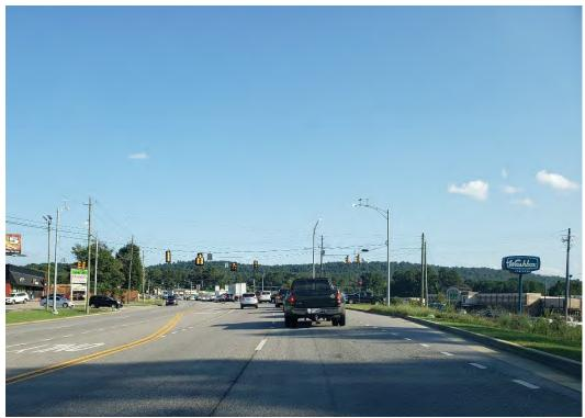
Figure 4: Congestion along SR-77 SB queued back from the US-411 intersection through the Independent Drive intersection during the PM peak hour
