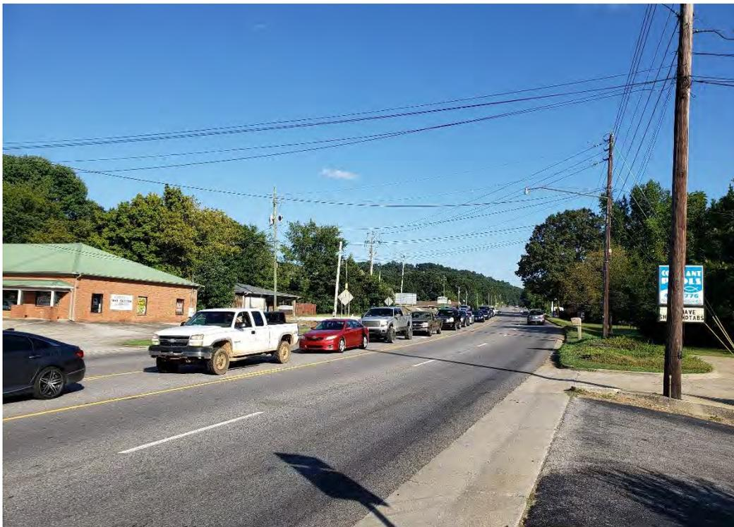
**Figure 5: Left turn traffic along SR-77 NB queued back from the US-411 intersection to the Church Street intersection during the PM peak hour**
