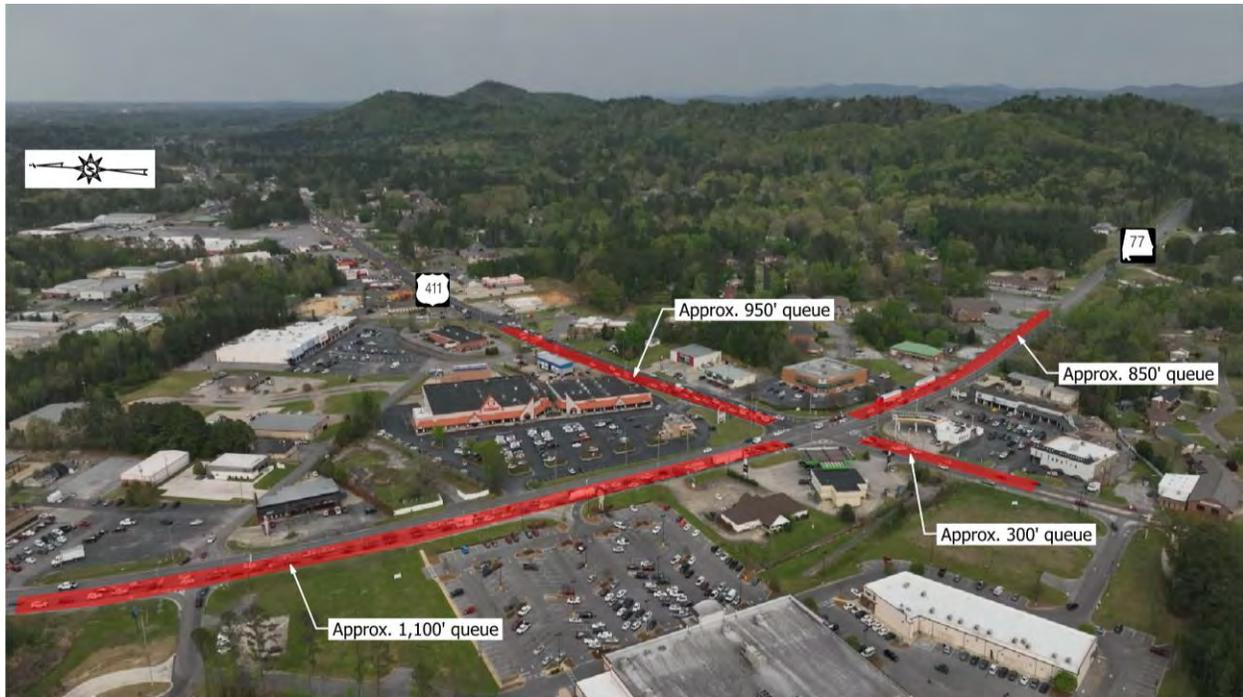
**Figure 6: PM Peak Hour Drone Observations**
