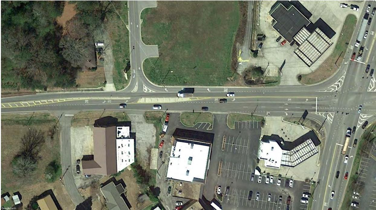
**Figure 27: Example of Access Management on US-411 near SR-77 Intersection**
